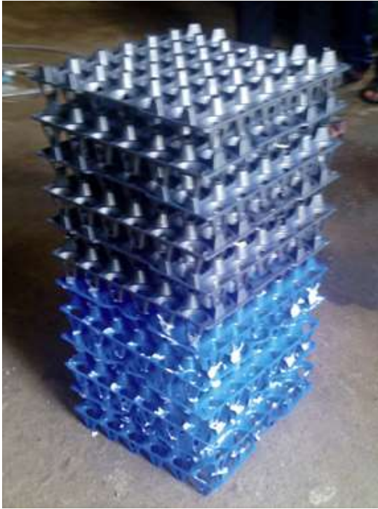
Plate 4: Arrangement of egg tray in the bio-filter water treatment tank
